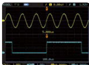
Alternate Trigger Provides a true dual time base display that was common in analog oscilloscopes
