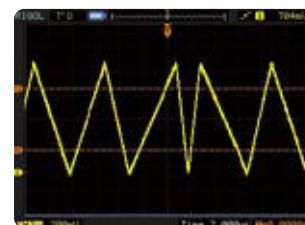
Slope Trigger Triggers on the signals rise time or fall time that is user defined
